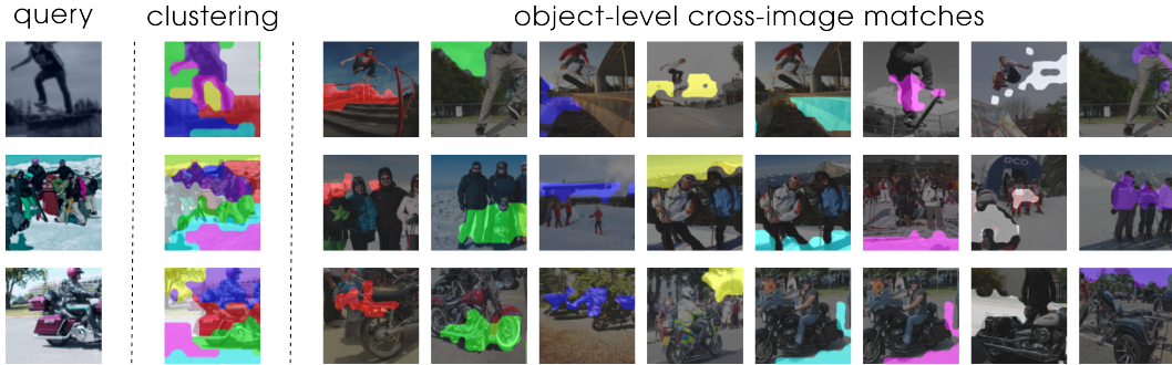
Figure 4: Visualization of cross-image object-level matchings on COCO. For a given query view (considered as view 1 here), object representations are computed via clustering. For each object-representation c_1^k (highlighted in unique colors), its nearest neighbor \text{nn}(c_1^k, \mathcal{M}_1) in the memory bank \mathcal{M}_1 is visualized. In this visualization, K = 12 .
