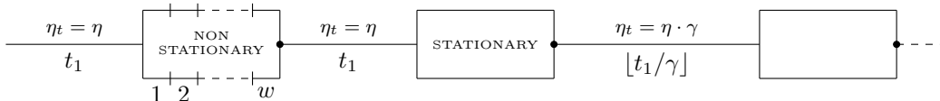
Figure 2: The architecture of SplitSGD. The initial learning rate is \eta and the length of the first single thread is t_1 . If the diagnostic does not detect stationarity, the length and learning rate of the next thread remain unchanged. If stationarity is observed, we decrease the learning rate by a factor \gamma and proportionally increase the length.
