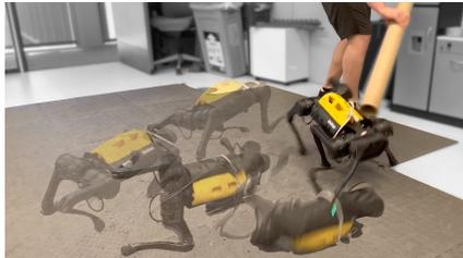
Figure 8: Within 10 minutes of perturbing the learned walking behavior, the robot adapts to withstanding pushes or quickly rolling over and back on its feet.
