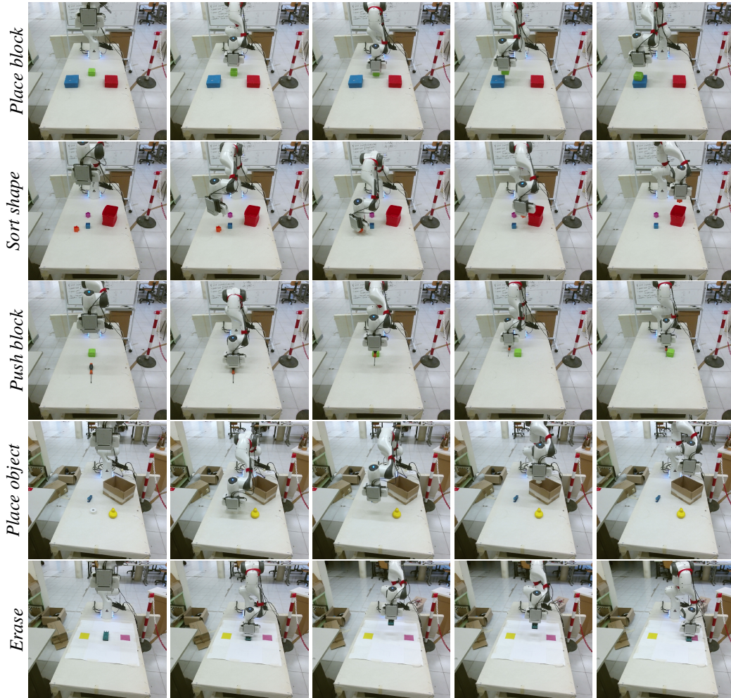
Figure F.9: Visualization of the real tasks. From top to bottom: place block , sort shape , push block , place object , erase .
