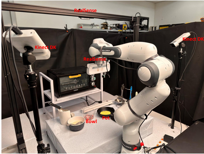
Figure 8: Our real-world scene with four cameras and a Franka Emika robot arm.
