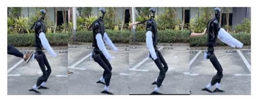
Figure 13: Robustness in Outdoor Settings: The robot responds to external disturbances in an outdoor environment by waving its arms and adjusting its gaits to maintain balance.
