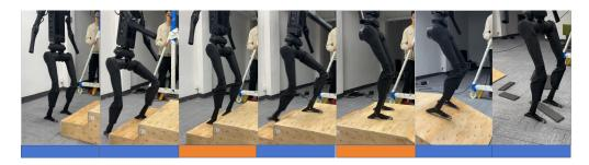
Figure 10: Climb Stairs Test. The blue segments indicate the activation of the goal-tracking policy, while the orange segments correspond to the safety recovery policy.
