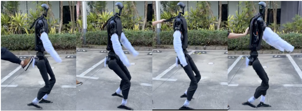
Figure 13: Robustness in Outdoor Settings: The robot responds to external disturbances in an outdoor environment by waving its arms and adjusting its gaits to maintain balance.
