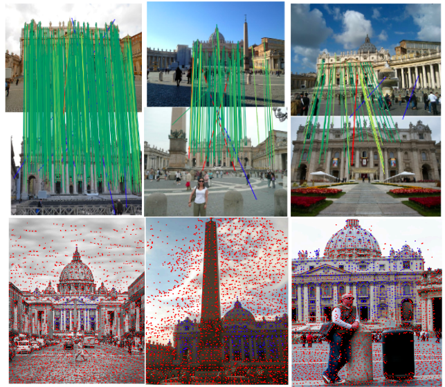
Figure 8: Visualization of correspondence for the stereo task and reconstruction points in the multi-view task. (green represents a correct match, yellow encodes a match error within 5 pixels, red shows the wrong match, blue shows the keypoints with the correct 3D points).
