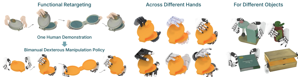
Figure 1: Functional Retargeting. We study the problem of functional retargeting, where the goal is to retarget human hand demonstrations into functional dexterous robot policies that manipulate an object to follow the demonstrated trajectory. Our proposed algorithm, DexMachina, achieves functional retargeting from one human demonstration to a variety of existing dexterous hand embodiments over a range of articulated objects.
