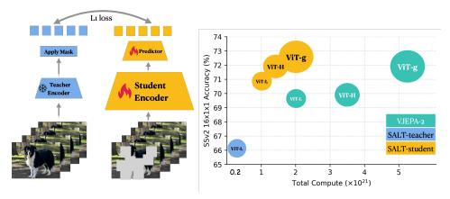
Figure 1: (Left) SALT Stage 2: Frozen-teacher, learnable student and predictor. The frozen teacher encoder is obtained via Stage 1 (not pictured above) by training using a pixel reconstruction objective. The student and predictor are jointly optimized to learn representation from video in Stage 2 using a latent space prediction objective. (Right): SALT's compute-accuracy curve dominates V-JEPA 2.
