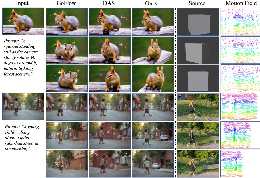
Figure 7: Qualitative comparison on unaligned control. DAS (Gu et al., 2025) introduces artifacts (red artifacts around the subject) from strict alignment, while Go-with-the-Flow (Burgert et al., 2025) produces implausible results. Our method flexibly follows input motion.
