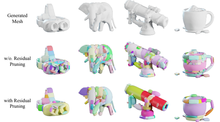
Fig. 11. Ablation on Residual Pruning. Since optimization-based fitting algorithms always try to fully occupy the interior of the input geometry, they tend to generate many fragmented superquadrics around the surface. Adaptive residual pruning effectively removes these fragments.
