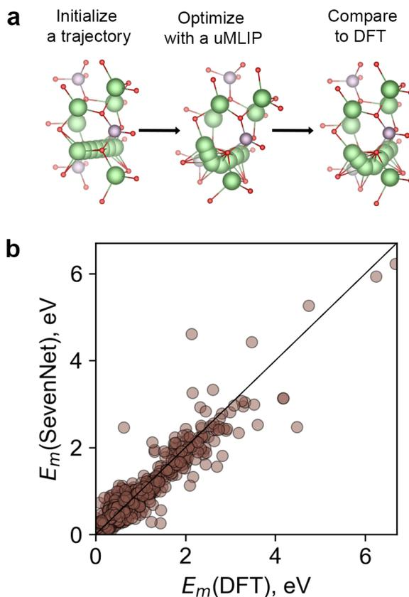
Fig. 1: a) A scheme for benchmarking uMLIPs on the nebDFT2k dataset, b) Parity plot for the predictions of the SevenNet model.
