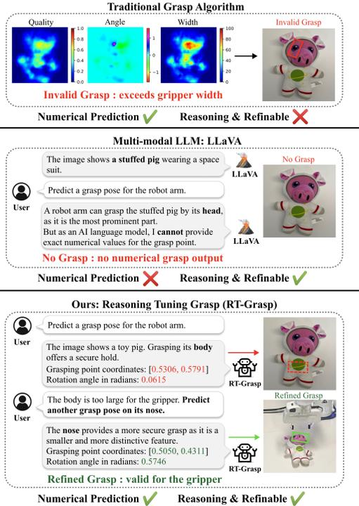
Figure 1: Comparing three robotic grasping approaches: 1) Traditional CNN-based algorithms produce fixed poses, which lack adaptability in practical situations. 2) Multi-modal LLMs output adaptable grasping strategies but lack precise numerical predictions. 3) Ours combines the best of both, predicting adaptable numerical grasping informed by reasoned strategies.
