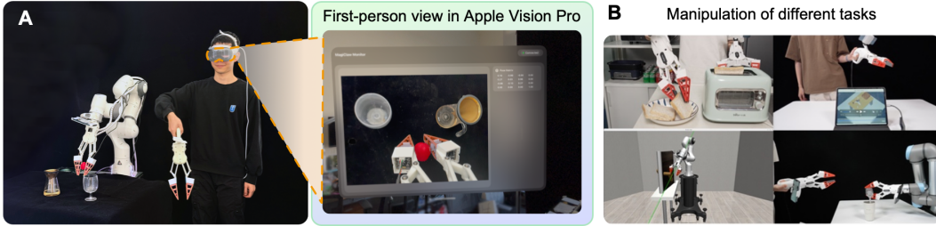
Figure 3: MagiClaw in Action. (A) An operator performs teleoperation with an immersive, first-person view provided by an Apple Vision Pro headset, which overlays real-time sensor data. (B) The system’s versatility is demonstrated across various manipulation tasks, both in the real world and in simulation, showcasing its adaptability.
