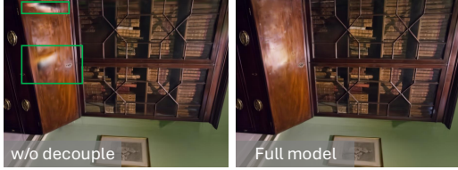
Figure 5: Ablation of decoupled neural fields. Using a single neural field to predict Gaussian properties causes gaps and holes.
