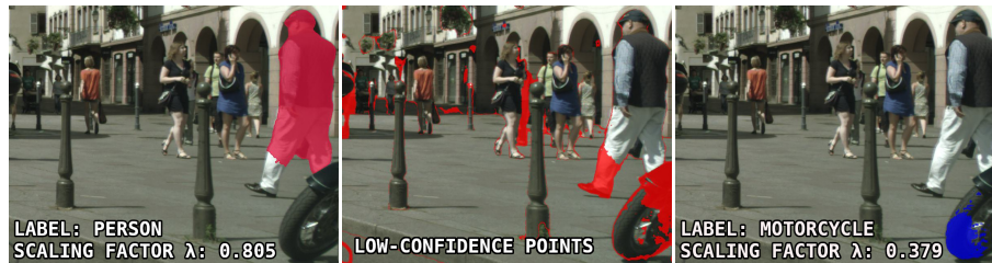
Fig. 6: Mask-wide loss-scaling and confidence-based point filtering exhibit complementary contributions to the selection of pixels for domain-adaptive learning. The central image highlights the two regions where back-propagation is withheld due to low teacher confidence. The other two images show that these two regions correspond to false negative pixels in the person mask (left) and the motorcycle mask (right).
