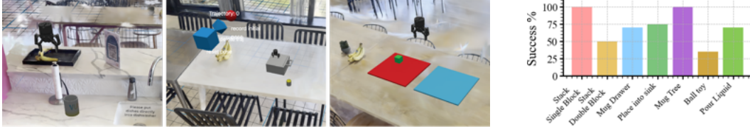
(a) Real-to-sim evaluation. We made 3D Gaussian scans of real-world kitchen environments to stage the evaluation environments, as a rough estimate of the generalization capability of the trained policy.
