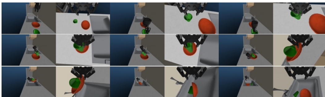
Figure 14: Cleaning The Kitchen. The robot learns to pick up a cup and stack it on top of the bowl, followed by placing both objects into the kitchen sink.
