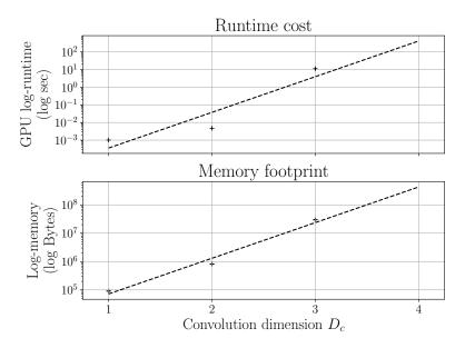
Figure 10: Scaling of the runtime cost and memory footprint of a CNN as a function of the convolution dimension. See text for discussion. *Error bars have been included for the runtime, but are too small to be seen in this plot.*
