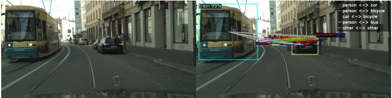
Figure 3. Qualitative results illustrating scale robustness in heterogeneous urban driving environments. The left panel represents the raw street environment. The right panel displays the corresponding CCFF inference result. Our model simultaneously maps the co-occurrences by utilizing a highly confident macro landmark (e.g., the 99% confidence train extraction) as a structural anchor. The co-occurrence links (e.g., yellow line represents person \leftrightarrow bus ) act as a contextual representation to confidently identify and recover distant or heavily occluded background instances.
