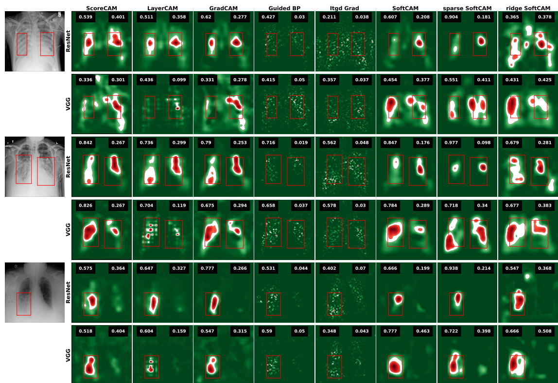
Figure 13: Localization precision and sensitivity for pneumonia detection. Each column shows explanations generated by different methods. Ground-truth bounding boxes are drawn on each map, with the top-right value indicating the activation precision, while the top-left value indicates the activation sensitivity. This shows the trade-off between ridge and lasso regularization.
