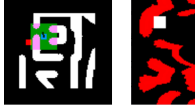
Figure 5: Dummy training environment (left) and the associated polar costmap (right).
