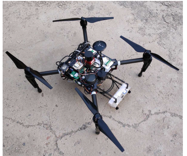
Figure 2. The device we used for our dataset. It contains oblique top-down global shutter stereo camera( AR0135, 30Hz) with 752×480 resolution and it contains a build-in IMU ( ICM20602, 500Hz ).
