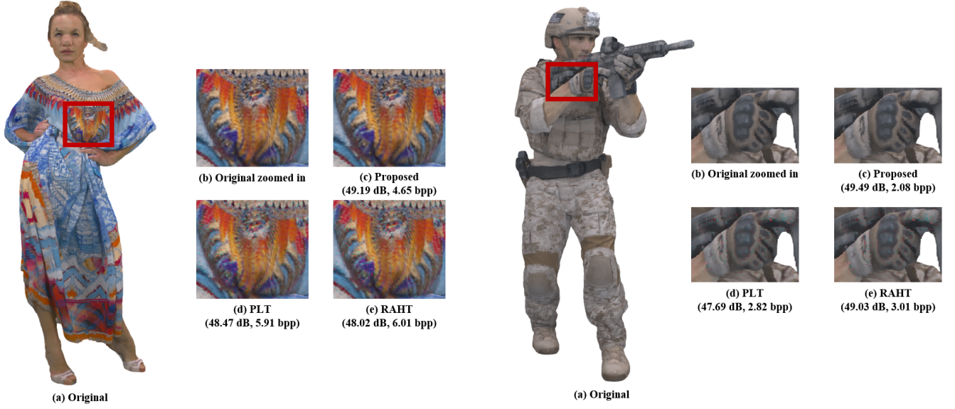
Figure 4: Visual quality comparison of the reconstructed longdress (left) and soldier (right) point clouds for proposed method, PLT and RAHT. Each sub-figure is annotated with corresponding bit rate (bpp) and distortion (dB).
