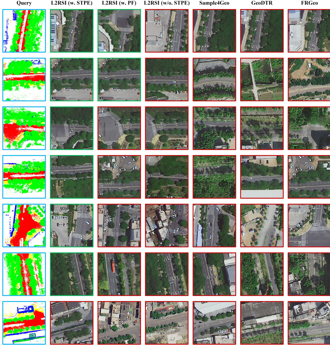
Figure 7: Qualitative comparisons on Test Set-G. Light blue boxes indicate the query point cloud submaps. Green boxes indicate correct retrieval results, while red boxes indicate incorrect results. To facilitate identification for the readers, we rotate the query to align with the same orientation as the remote sensing imagery.
