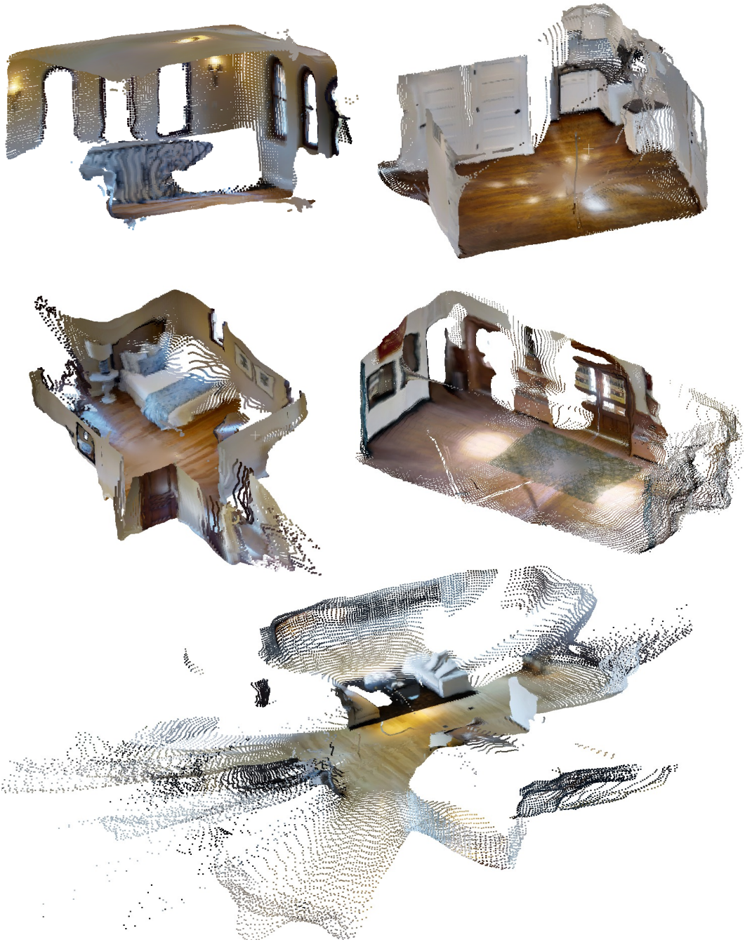
Figure 11: 3D geometry of Matterport3D using matches and certainties produced by EDM. These point clouds result from spherical triangulation with estimated poses between two omnidirectional images.
