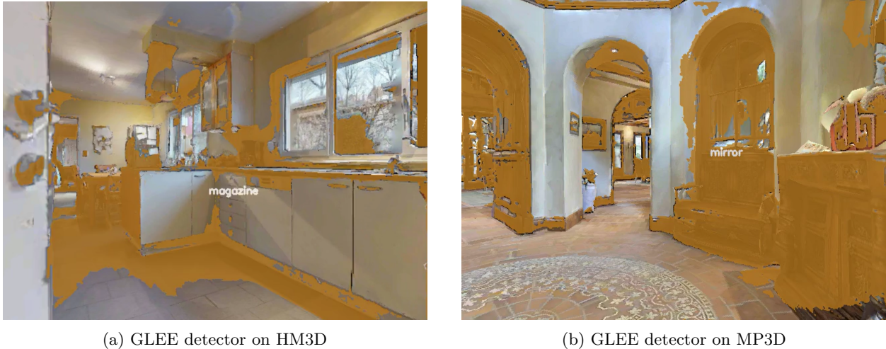
Figure 3: Failure modes of the open-vocabulary segmenter used in InstructNav. Typical cases include no detections under indoor lighting/texture and near-image-wide false positives on stylized surfaces. These errors corrupt the semantic value map and can mislead downstream planning. Our use of a ground-truth semantic sensor for the fairness control (InstructNav-GT) prevents such noise in the baselines used for comparison.
