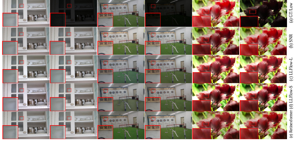
Figure 4: Quantitative comparison of LOL-v1 [53] (1st–2nd columns), LOL-v2-real [65] (3rd–4th columns), and LOL-v2-syn [65] (5th–6th columns). Even columns correspond to the results of adding the TTS module.
