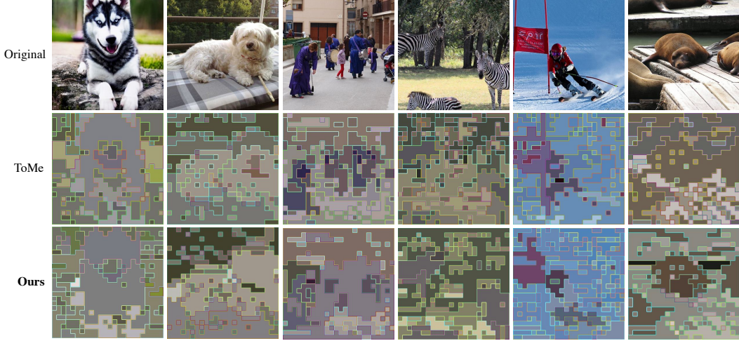
Figure 5: Qualitative comparison of DSM to ToMe using a ViT-L 384 model. Merged tokens share the same border and filling color. DSM merges more contiguous patches that are semantically similar, leading to more interpretable outcomes that retain the original features. For example, the skier’s legs are merged with the background in ToMe, while DSM provides correct segmentations.
