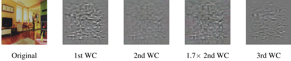
Figure 3: Visualisation of the restoration process in the case of TrustMark. The first watermark component (1st WC) is 10\times the subtraction between the watermarked image and the original image, the second watermark component (2nd WC) is 10\times the subtraction between the double watermarked image and the watermarked image, and the third watermark component (3rd WC) is the subtraction between the restored image and the original image. The optimum scale factor is 1.7.
