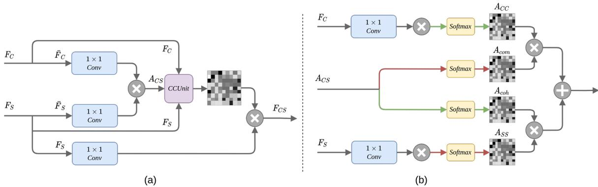
Figure 17: (a) Architecture of the lightweight Non-local Diffusive Attention Module. (b) Architecture of our CCUnit which captures completeness and coherence at once. Please refer to Sec. C for details.
