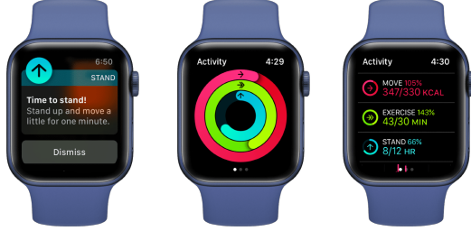
Figure 1: (Left) The standing notification is delivered at 6:50 pm because the user didn’t stand from 6:00 pm to 6:50 pm. (Middle) The Apple Watch activity Rings that users are encouraged to close each day. (Right) Details of the goals that a user need to reach to close each of the three rings: number of active calorie burned for the Move ring in red, number of exercise minutes for the Exercise ring in green and number of hours containing at least one minute of standing for the Stand ring light blue.
