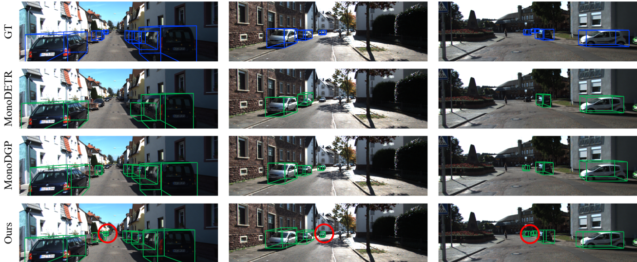
Figure 6. Visualization of comparative results on the KITTI val set. Blue boxes: ground truth annotations; Green boxes: detection results from different methods; Red circles: performance advantages of our method over competing approaches.
