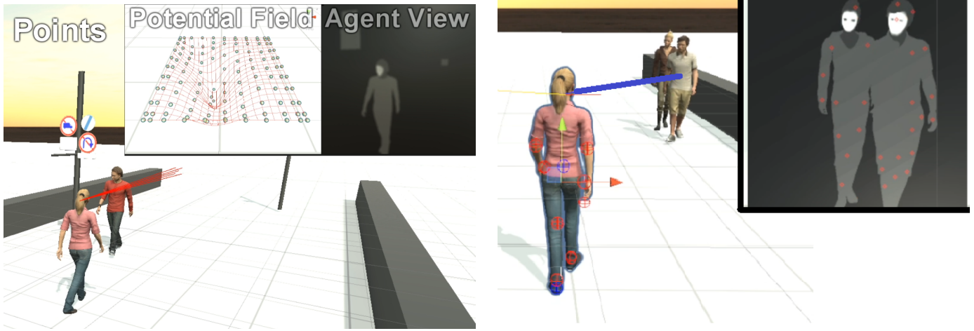
Figure 5: Comparison of target selection between the two models. Left: Particle model, which drives gaze in the direction of the potential field gradient. Right: Probabilistic model target selection. Red circles indicate potential target locations, which once selected will trigger a saccade.
