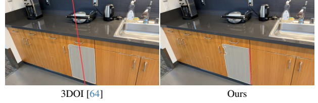
Figure 3. Articulation Estimation: We visualize the estimated revolute axes and articulated object masks produced by 3DOI [64] and DRAWER, demonstrating that DRAWER achieves more precise articulation estimation due to its underlying 3D geometry.
