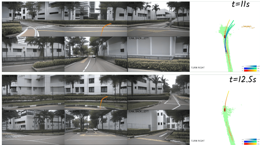
Figure 14: Failure cases of UniAD in DRIVEARENA’s closed-loop mode. While UniAD generally predicts road structures accurately: (top) UniAD encroaching onto the central median; (bottom) UniAD failing to complete a right turn successfully.
