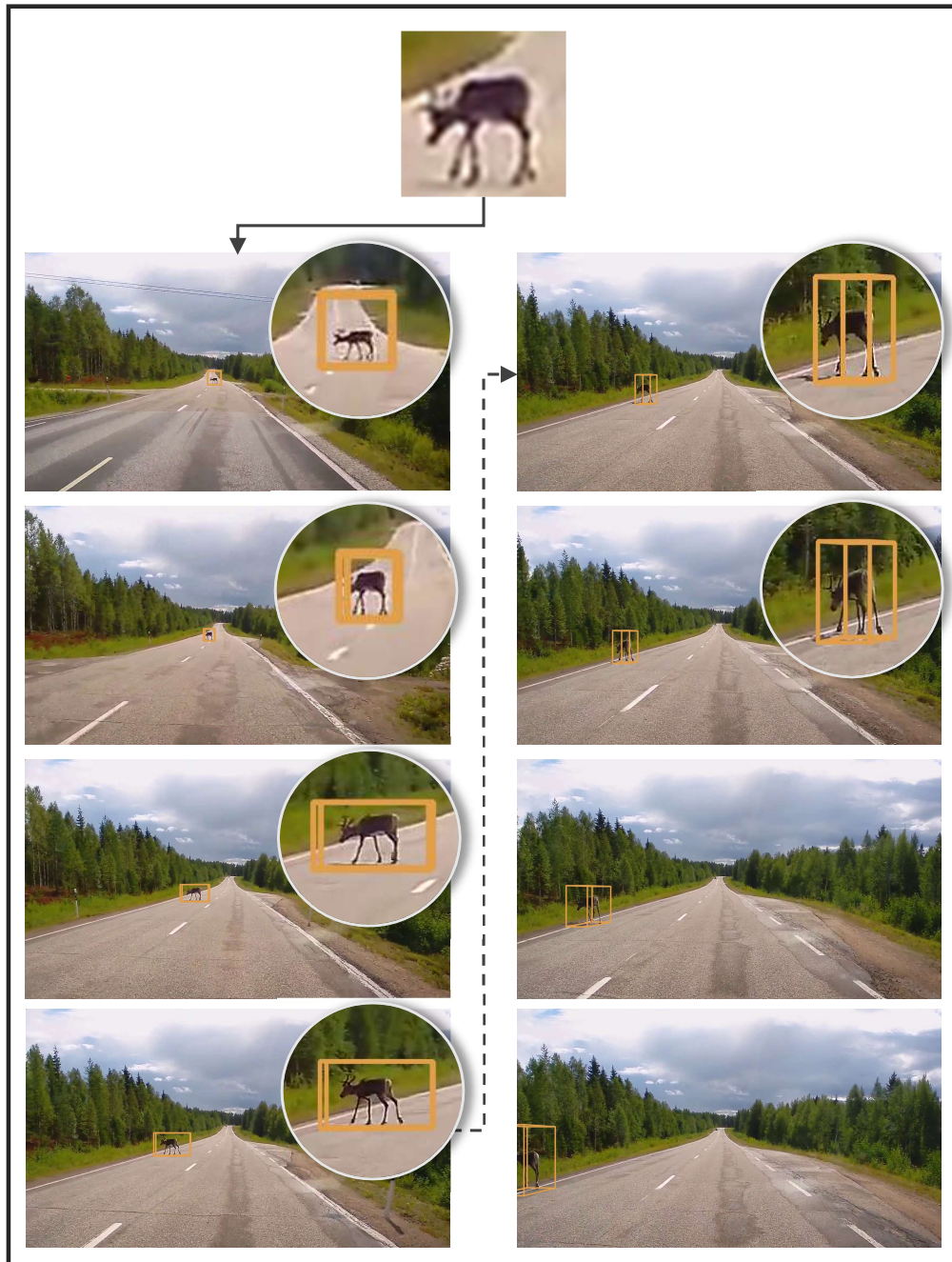
Figure 23: Visualizations on real world scenarios with out-of-domain visual prompts. This figure demonstrates a case of real-world 3D object detection. We provide the visual prompt from the same scene as the target object, though it is unseen during training, and our TTC system then detects the target objects in the subsequent video frames.
