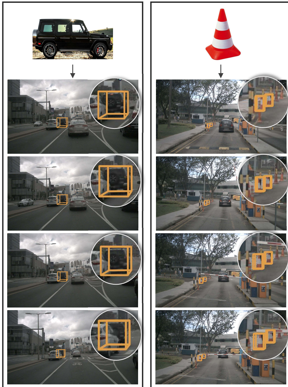
Figure 18: Visualizations on nuScenes scenarios with out-domain visual prompts of labeled objects. TTC system can perform 3D detection and tracking via visual prompts with arbitrary styles ( imagery style ). The image in the first row indicates the visual prompt in the prompt buffer, and images in other rows represent 3D detection results prompted by the corresponding visual prompts. With the one-to-N mapping mechanism of the visual prompt alignment, TTC detectors can detect multiple objects with similar visual descriptions to the visual prompt at the same time.
