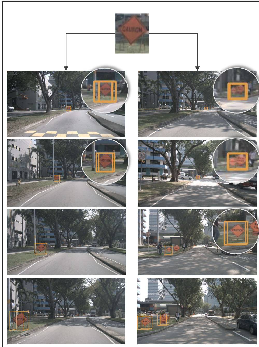
Figure 17: Visualizations on nuScenes scenarios with in-domain visual prompts of un-labeled objects. TTC system enables 3D detection and tracking of “novel” objects unseen during training. The image in the first row indicates the visual prompt in the prompt buffer, and images in other rows represent 3D detection results prompted by the corresponding visual prompts. Interestingly, with the one-to-N mapping mechanism of the visual prompt alignment, TTC system can detect multiple objects with similar visual descriptions to the visual prompt simultaneously.
