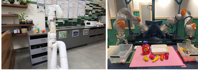
Figure A3: (Left) Office kitchen environment with drawers and bins for the Mobile Manipulation setting. (Right) Bimanual setup with the set of objects used in the experiments.
