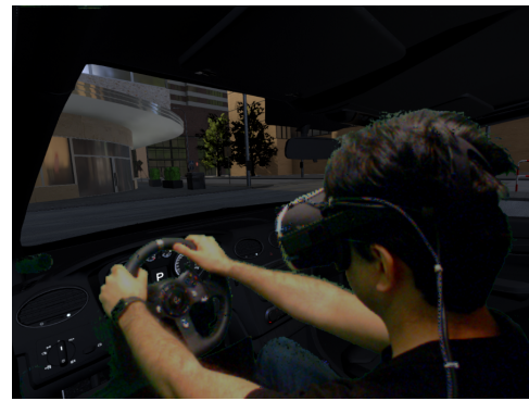
Figure 4: A third-person view of a user driving the simulator in front of a green screen, composited with the virtual vehicle.
