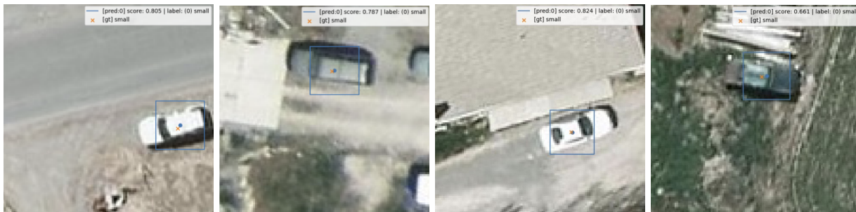
Figure 5: YOLOv5 Detection Visualization, where the orange X is the ground truth annotation, and the blue dot with the bounding box is the prediction result.
