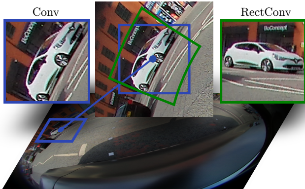
Figure 2: An example of what regular convolution and RectConv see for a fisheye image at a given position in the image. Blue and green boxes indicate the kernel shapes for regular convolution and RectConv, respectively.
