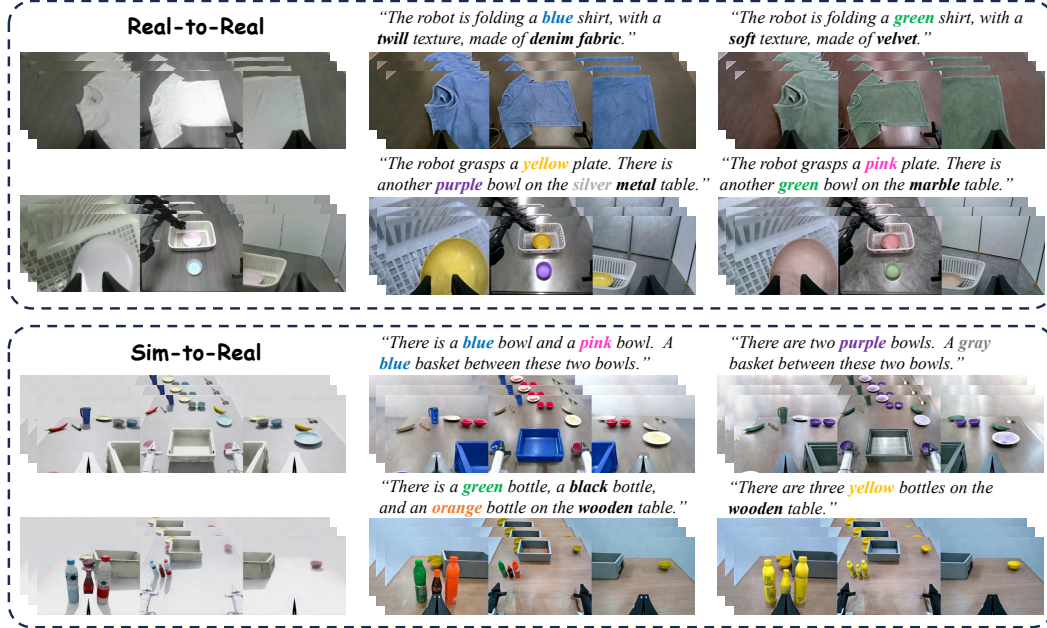
Figure 1: DreamTransfer demonstrates strong controllability in embodied manipulation video generation. It excels in text-controlled appearance editing while preserving 3D structure and geometric plausibility, and supports both real-to-real and sim-to-real transfer. The complete prompts used for generation is provided in the supplementary materials.
