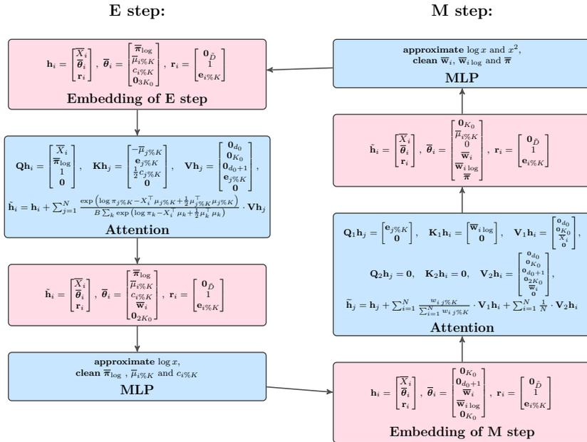
Figure 9: Transformer Construction for Approximating EM Algorithm Iterations. The *pink box* represents the state of tokens, while the *blue box* represents the structure of different parts of the network. The term "clean" means setting all positions of the corresponding vector to zero.
