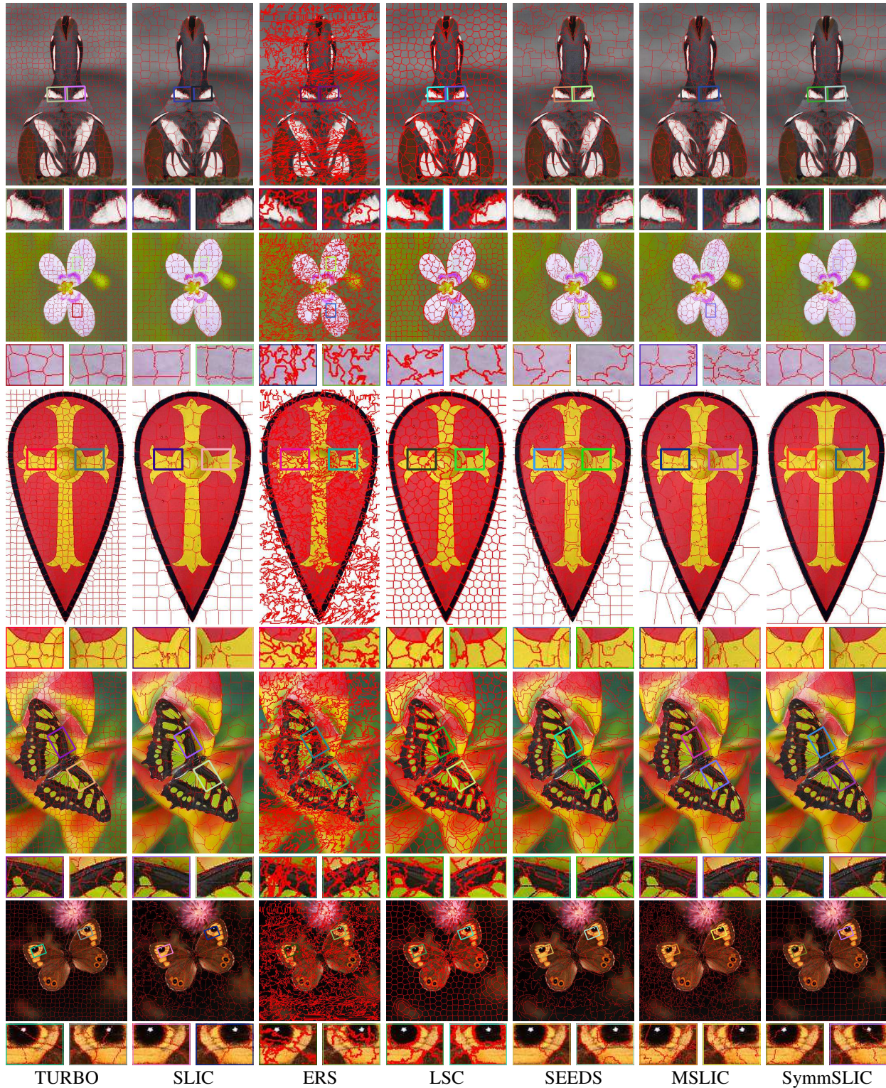
Figure 7. Results for the approaches TURBO [17], SLIC [1], ERS [19], LSC [18], SEEDS [52], MSLIC [22], and the proposed method. For each image, we show two zoomed-in mirror symmetric windows to visualize whether the superpixels are mirror reflections of each other or not. Window border represents its location in the image. The tilted windows are aligned horizontally.
