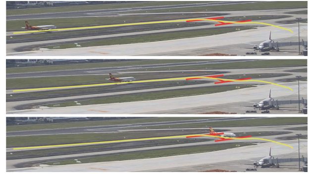
Fig. 13. Comparison between the manual annotation (red line) and the real trace of the moving aircraft (yellow line).
