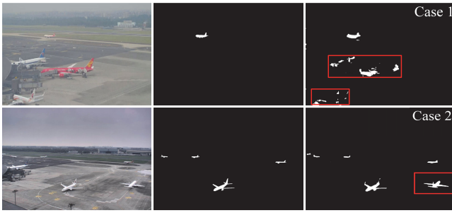
Fig. 2. The left column includes two frames extracted from the Airport Ground Video Surveillance (AGVS) dataset. The middle column includes the ground truth representation of moving objects. The right column includes the background subtraction outcomes generated by the Foreground Segmentation Network (FgSegNet) [4]. The AGVS dataset is specifically designed for airport background subtraction tasks, while FgSegNet operates on an encoder-decoder architecture. It's worth noting that FgSegNet erroneously identifies stationary aircraft (highlighted in red boxes) as foreground objects.
