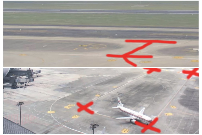
Fig. 7. Illustration of manually annotated turning areas in the flight zone and apron. When the aircraft passes through a turning area, the motion pattern, especially the direction, will change dramatically, while there is good motion consistency in the non-turning area. Therefore, only performing motion accumulation in the non-turning area can ensure the effectiveness of the accumulated features.
