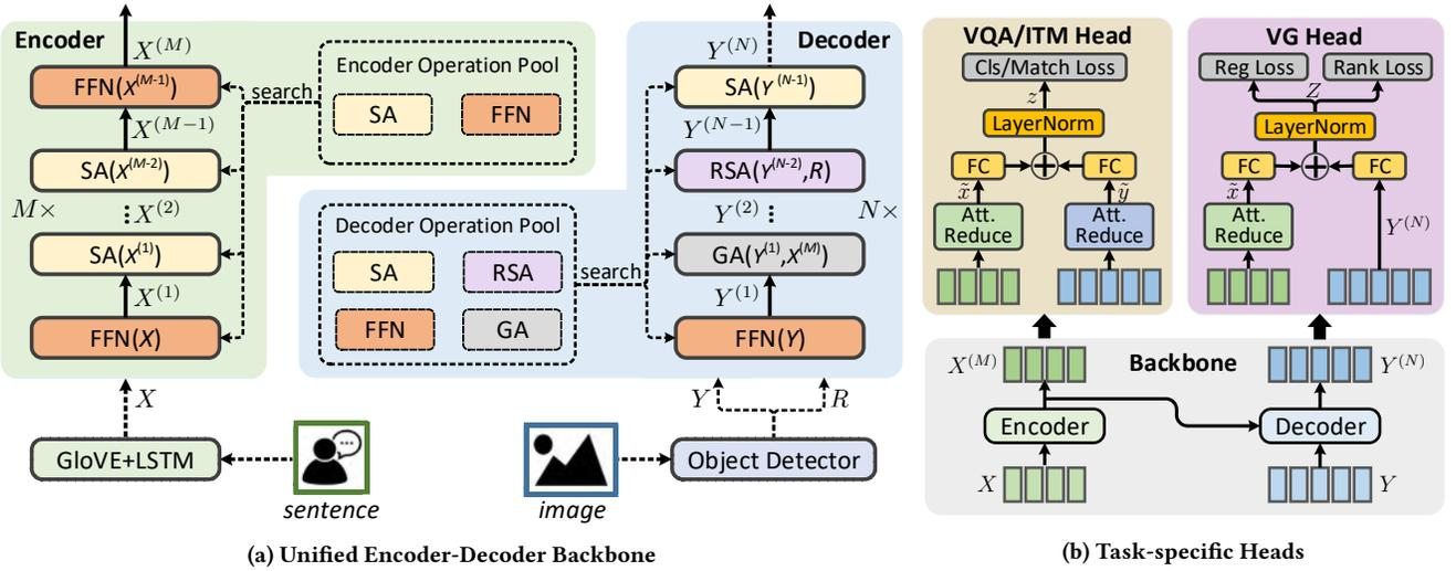
**Figure 2: The flowchart of the MMnas framework, which consists of (a) unified encoder-decoder backbone and (b) task-specific heads on top the backbone for visual question answer (VQA), image-text matching (ITM), and visual grounding (VG).**
