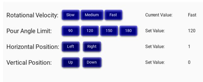
**Figure 4: Screenshot of the control panel used to adjust the parameters of the robot's pouring behavior .**
