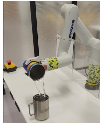
**Figure 1:** The robot used in our study, shown pouring water from a source to target container. In our experiments, participants were first tasked with predicting the outcome of a pouring action (spill vs. no spill). Participants were also tasked to adjust the parameters of the pouring action to minimize spills.
