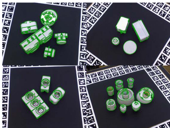
Fig. 14. Qualitative results for T-LESS dataset, where the green edge line is a visualization of our predicted pose.
