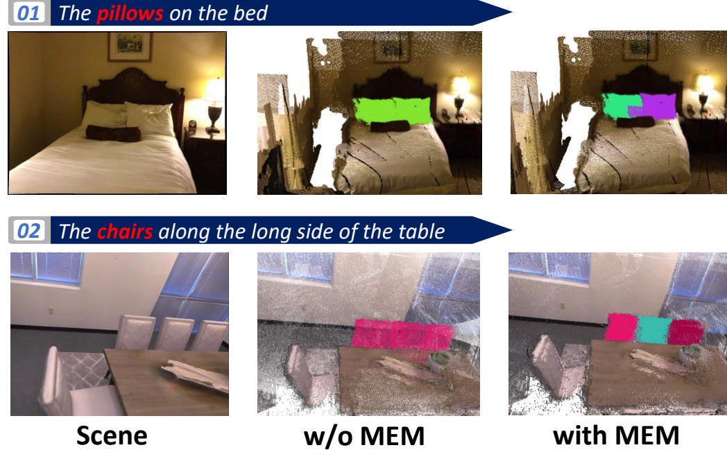
834 Figure 4: Qualitative ablation study of the MEM metric. When the MEM mechanism is absent, SLAM matching errors and mask under-segmentation often cause different objects that are adjacent in the scene and share the same semantic label to be merged into a single instance, such as side-by-side pillows or chairs. When the MEM mechanism is enabled, these adjacent objects with the same semantics can be correctly separated and reconstructed as independent instances.
