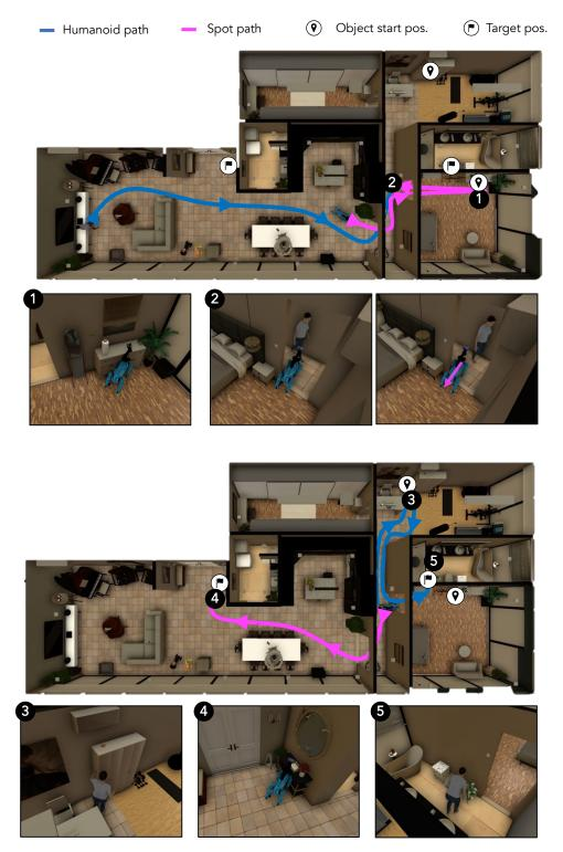
Figure 10: **Social Rearrangement Example**: We show an example behavior from the Plan-Pop<sub>3</sub> baseline with learned low-level skills. Here, the agents split the rearrangement task, with each picking one of the objects (frames 1, 3) and placing them in their target location (frames 4, 5). In frame 2, we observe an emergent collaborative behavior: the robot moves backward to let the humanoid pass through the hallway, before continuing with its task, avoiding a collision.
