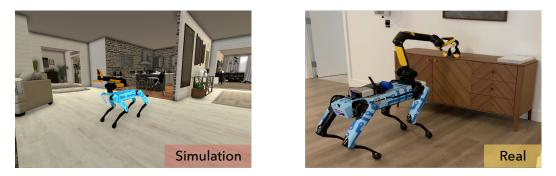
Figure 9: **Robot Embodiment.** Spot robot in the simulation environment is designed to minimize the embodiment gaps to the robot in the physical world.
