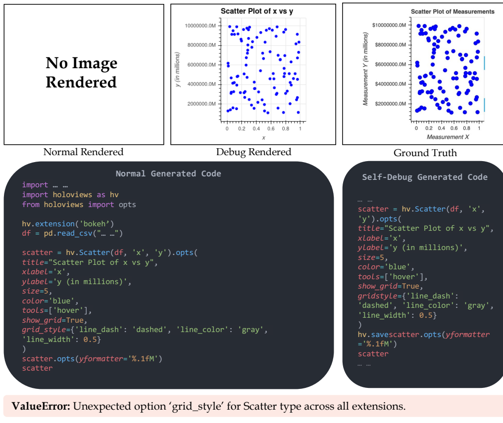
Figure 6: Example of a failed generation in Python (ID: 69), where the initial code raises a ValueError and is resolved in the first round of self-debug, resulting in a corrected plot that matches the intended semantics.
